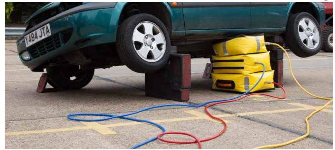
MFC Survival offer a 2 or 3 tier of low pressure Airlift cushions designed primarily for the recovery of vehicles. These cushions have a large contact area which means they uniformly distribute lift pressure across a large surface area, making them suitable for lifting at weak points of a vehicle such as the roof, sides, wings, bonnet and boot.
